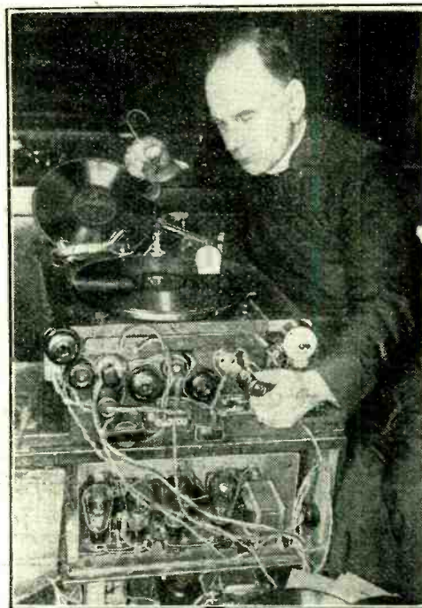
RINGING THE CHANGES.—The Rev. Isa Rees-Jones, vicar of Yardley Wood, Birmingham, has constructed this 50-watt amplifier in his study for the reproduction of chimes on three loud speakers mounted in the church tower, 500 yards away.
